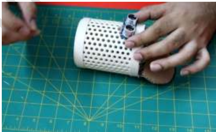
Figure 9: Attach the ultrasonic sensor with dustbin
