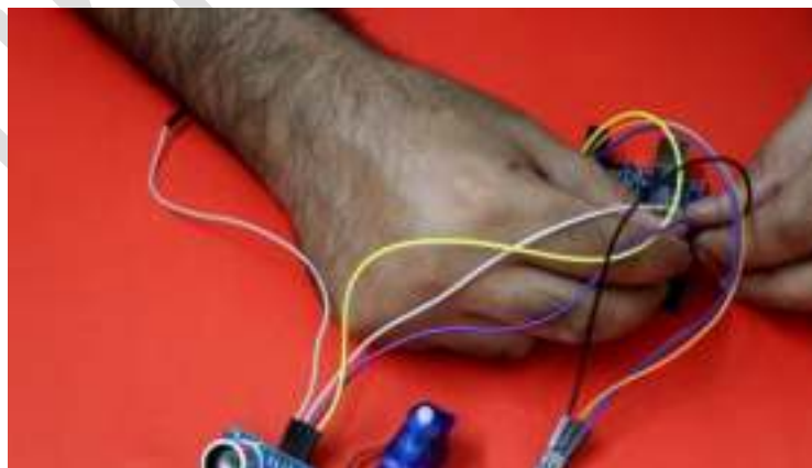
Figure15: Connect one end of the white wire with pin “D#6” on Arduino and another end with pin “Echo” on ultrasonic sensor
