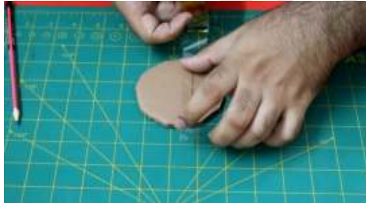
Figure 5: Connect part A and B of cardboard using paper tape
